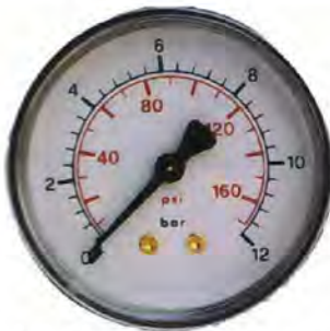
M C 50...: \varnothing 50 Axial pressure gauge ( available scale in bar: 4, 6,10,12,16 Bar) 1/4" GAS connection- Back entry - Copper tubular spring – Sn-Ag welding - Working temperature: -20°C / +80°C – box: black plastic
