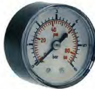
M R 63... \varnothing 63 Axial pressure gauge ( available scale in bar: 4, 6,10,12,16 Bar) 1/4" GAS connection- Back entry - Copper tubular spring – Sn-Ag welding - Working temperature: -20°C / +80°C – box: black plastic
