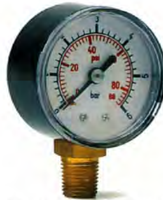
M R 63...Radial pressure gauge \varnothing 63 ( available scale in bar: 4, 6,10,12,16 Bar) ) 1/4" GAS connection- Bottom entry - Copper tubular spring – Sn- Ag welding Working temperature: -20°C / +80°C – box: black plastic
