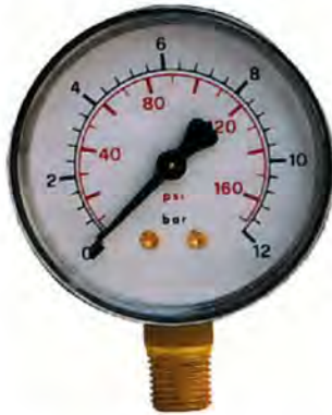
M R 50...: Radial pressure gauge \varnothing 50 ( available scale in bar: 4, 6,10,12,16 Bar) 1/4" GAS connection- Bottom entry - Copper tubular spring – Sn-Ag welding - Working temperature: -20°C / +80°C – box: black plastic
