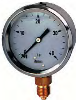
M GX ... : Pressure gauge with glycerine \varnothing 50., 63 or 100 ( available scales in bar: 4, 6,10,12,16, 20,25,40 e 100 Bar)1/4" GAS connection ( 1/2" connection for r \varnothing 100) Bottom entry (M GX ...R) or back entry ( M GX C) – Working temperature: -10°C / +80°C – STAINLESS STEEL CONSTRUCTION
