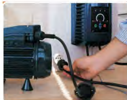
5) Connect the Inverter to the mains
