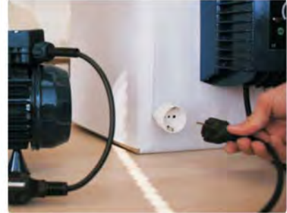
2) Disconnect the feeding cable From the mains
