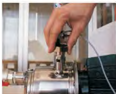
3) Install the pressure trasducer
