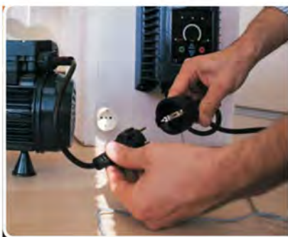
6) Connect the inverter to the Electric pump
