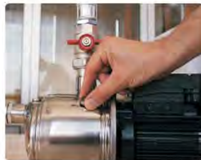
2) Remove the drain plug on the Pump casing
