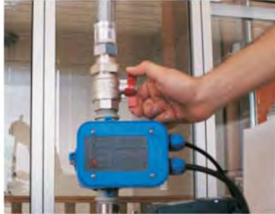
1) Close the delivery outlet regulator
