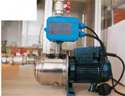
Old system controlled by pressure regulator
